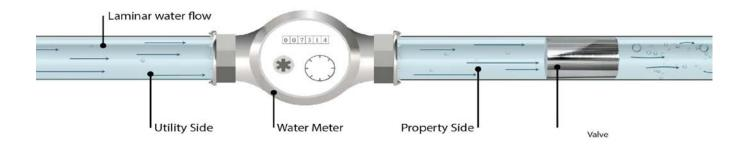
The SOLID DEW SMART Valve acts as a restrictor with a minimum reduction of 5%. The system reduces from a certain diameter to a smaller diameter, running for just 3mm before opening to a full port (95%). On the other side (proprietary), there is no significant effect on flow or pressure. This process is very similar to the Venturi effect.
